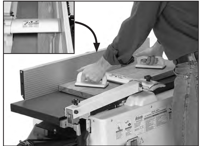
Figure 33. Surface planing board less than 3" thick.
